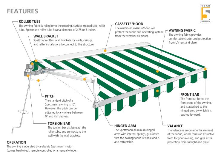
Spettmann awnings & shades are made with only the finest material and the highest quality workmanship. With top of the line powder-coating and hardware made with the highest grade stainless steel.
